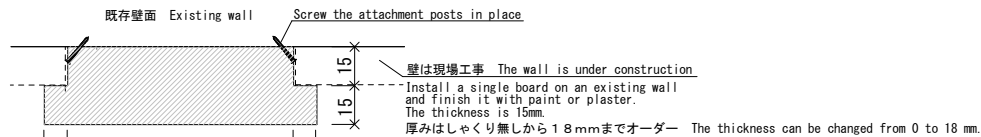
付け柱詳細図 scale1/2 Detail drawing of the attached column scale 1/2
